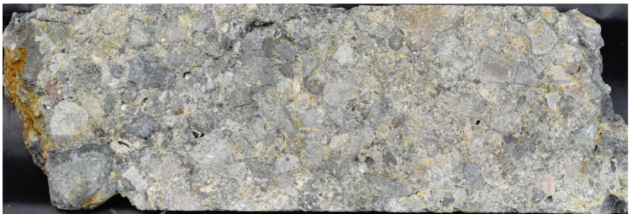
Figure 6: FDD004: Detailed core photograph of the interval from 82.40 to 82.60m (20cm). Polymictic breccia sub-rounded, clast supported, strong pervasive silica-clay-pyrite alteration, fine grain pyrite filling the matrix and disseminated in the clasts. 82 to 83m assayed 2.07g/t Au & 0.02% Cu .
