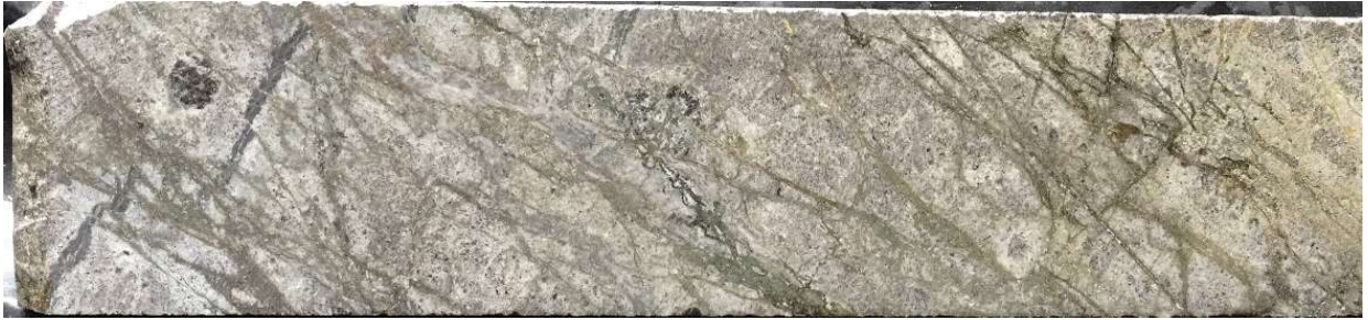
Figure 7: FDD004: Detailed core photograph of the interval 384.70 to 385.00m (30cm). Pervasive secondary biotite-magnetite-actinolite alteration overprinted with clay-silica-pyrite, fine to medium grain intrusive unit. Fine sulphides (pyrite + chalcopyrite) filling fractures/veinlets as well as disseminated. 384 to 385m assayed 1.84g/t Au & 0.34% Cu .
