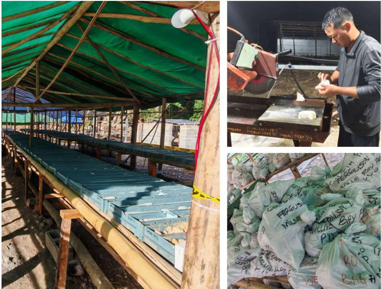
Figure 11-1 Core shed, core saw and sample despatch at Gameta during the 2025 drilling campaign
