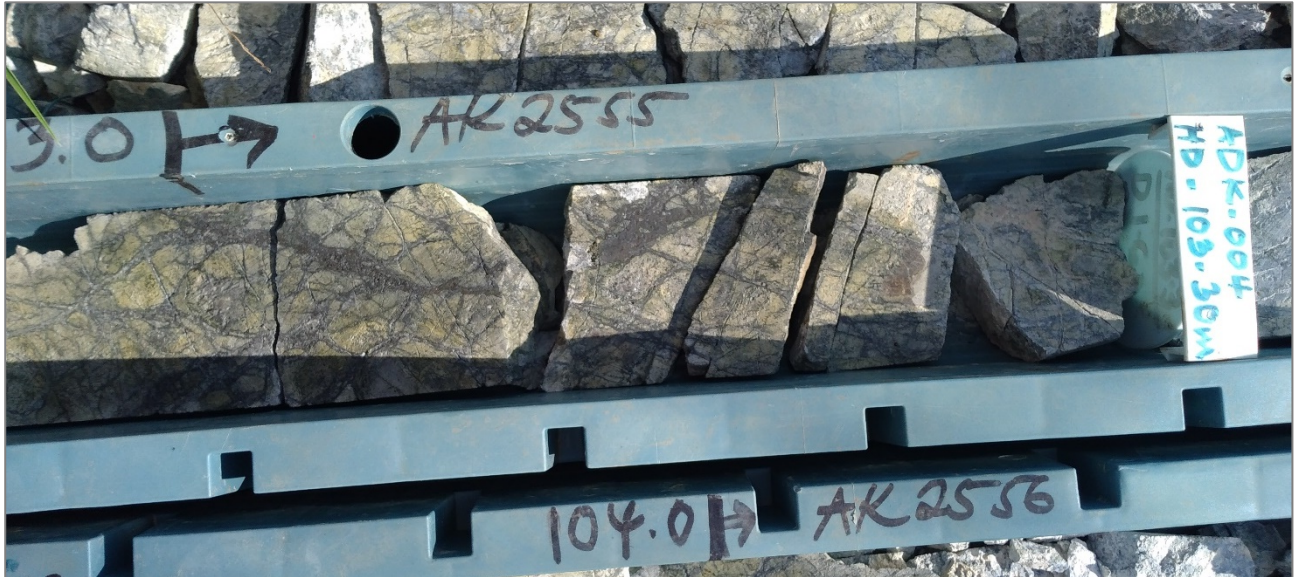
Figure 12-5. ADK004: 103.0 – 103.3 m, showing close-up of hydrothermal breccia, October 2021.
