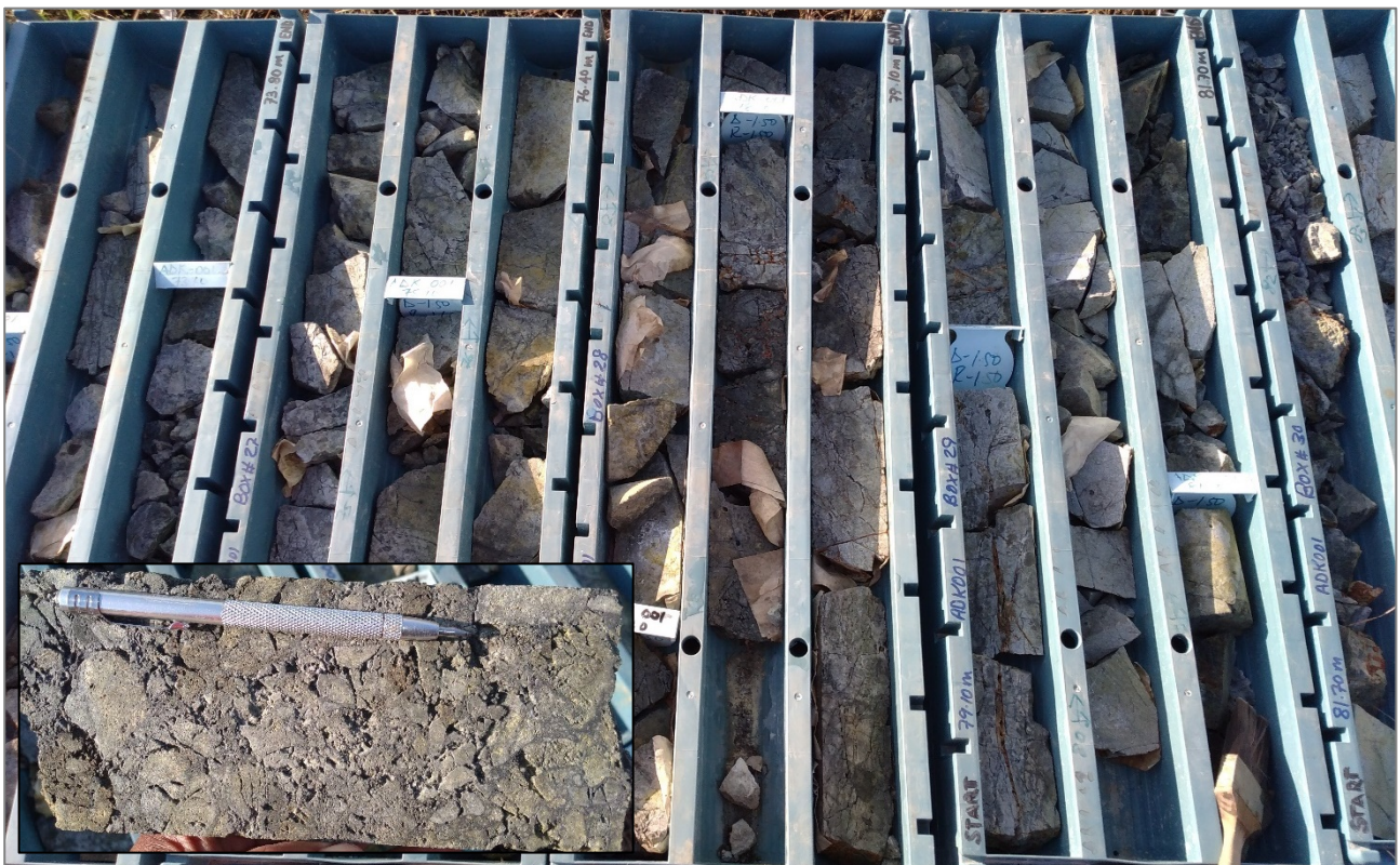
Figure 12-4. ADK001: 73.5 – 82.5 m, with inset showing close-up of breccia, October 2021.
