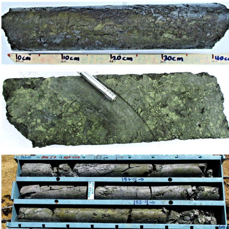
Figure 5: ADK004 – 155.1 – 156.1m showing massive sulphide mineralization in hydrothermal breccia
