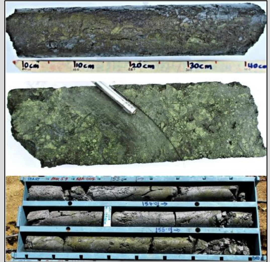
ADK004 – 155.1 – 156.1m Massive sulphide mineralization in Hydrothermal Breccia
