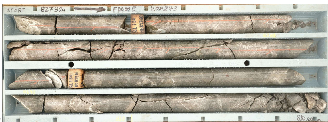
Figure 6: FDD005 Box 243 From 827.30m to 830.60m: monzodiorite with pervasive potassic (biotite+/k-feldspar) alteration, quartz+/-magnetite+/-pyrite/chalcopyrite veining and disseminated pyrite (3%) and chalcopyrite (1%) (assays pending).
