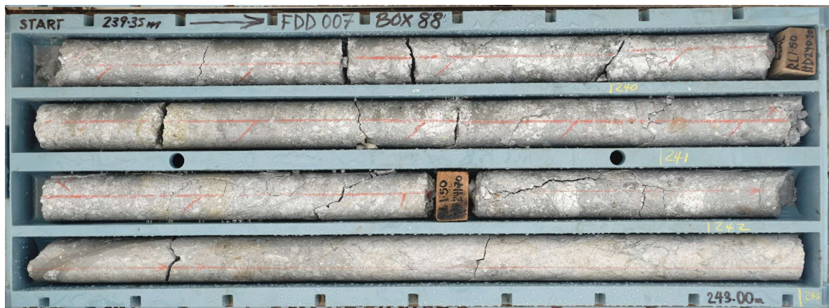
Figure 8: FDD007 zone proximal to 240m. Strongly sulphide-silica-clay altered and mineralised breccia (ca. 5-10% py-asp) (assays pending).
