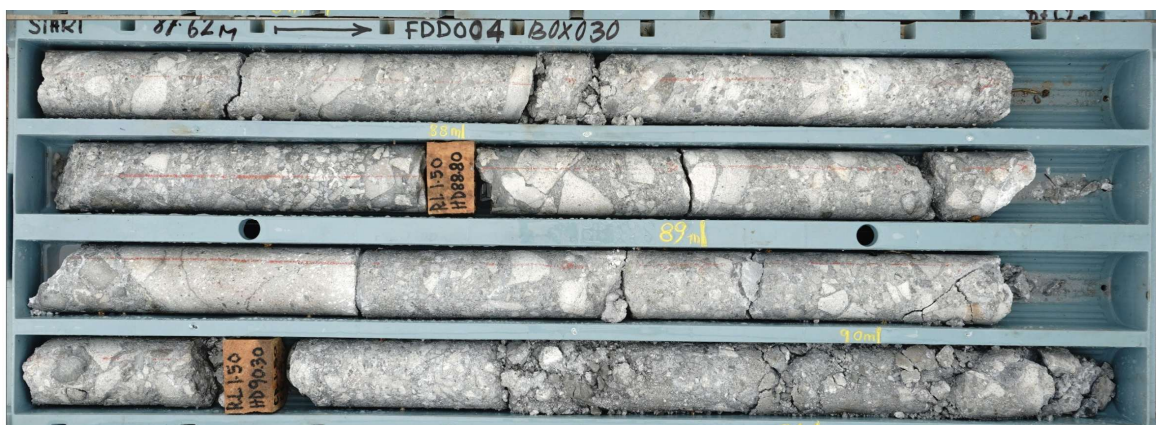
Figure 4: FDD004 from 87.62m to 91.2m. Sulphide (pyrite 5%) mineralized breccia (assays pending).
