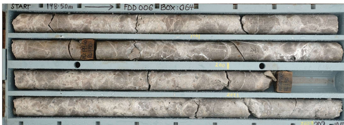
Figure 7: FDD006 from 198.5m to 202.10m. Potassic altered intrusive with stockwork qz-anhydrite veining with pervasively disseminated fine sulphides (pyrite 3%) (assays pending).
