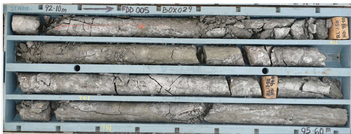
Figure 5: FDD005 from 92.10m to 95.60m. Semi-massive sulphide (5-10% pyrite-arsenopyrite-chalcopyrite) (assays pending).
