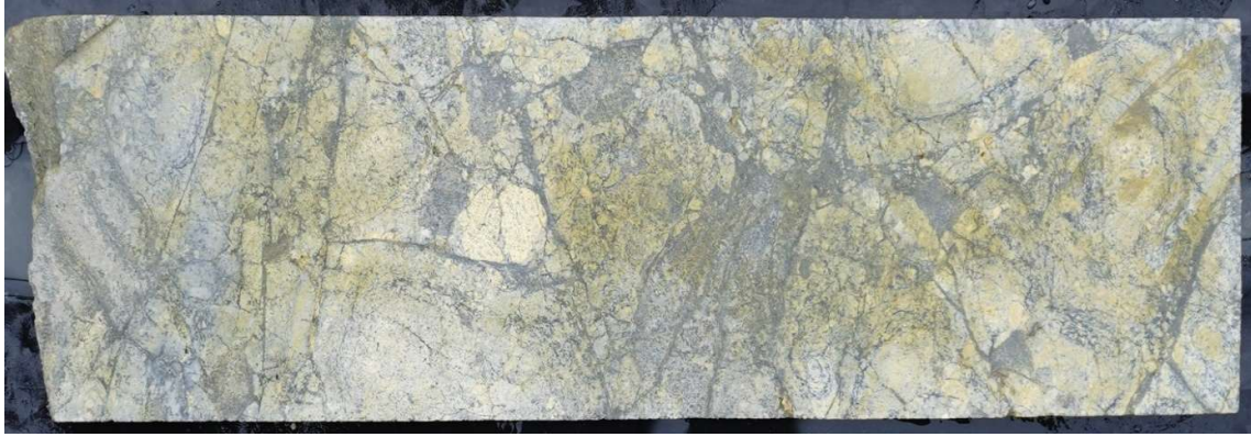
Figure 3: FDD001: Detailed core photograph of the interval from 107.3 to 107.6m (30cm). Crackle breccia within monzodiorite, sub-rounded, clast supported, strong pervasive silica-clay-pyrite alteration, fine grain pyrite filling the matrix and filling cracks and disseminated in the clasts. 107 to 108m assayed 3.91g/t Au & 0.02% Cu .
