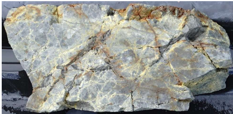
Figure 5: FDD003: Detailed core photograph of the interval 122.80 to 123.00m (20cm). Pervasive silica-clay-pyrite altered, fine to medium grain intrusive unit. Fine sulphides (pyrite + chalcopyrite) filling fractures as well as disseminated. 122 to 123m assayed 1.59g/t Au & 0.71% Cu .
