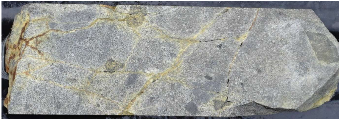
Figure 4: FDD002: Detailed core photograph of the interval from 112.10 to 112.30m (20cm). Pervasive silica-clay-pyrite altered, sub-round clasts set in fine to medium grain intrusive unit with fine disseminated pyrite. 112 to 113m assayed 2.36g/t Au & 0.04% Cu .
